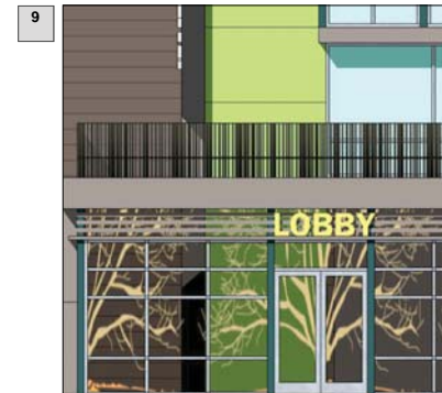
DECORATIVE WINDOW FILM (BLDG B NORTH ELEVATION)
