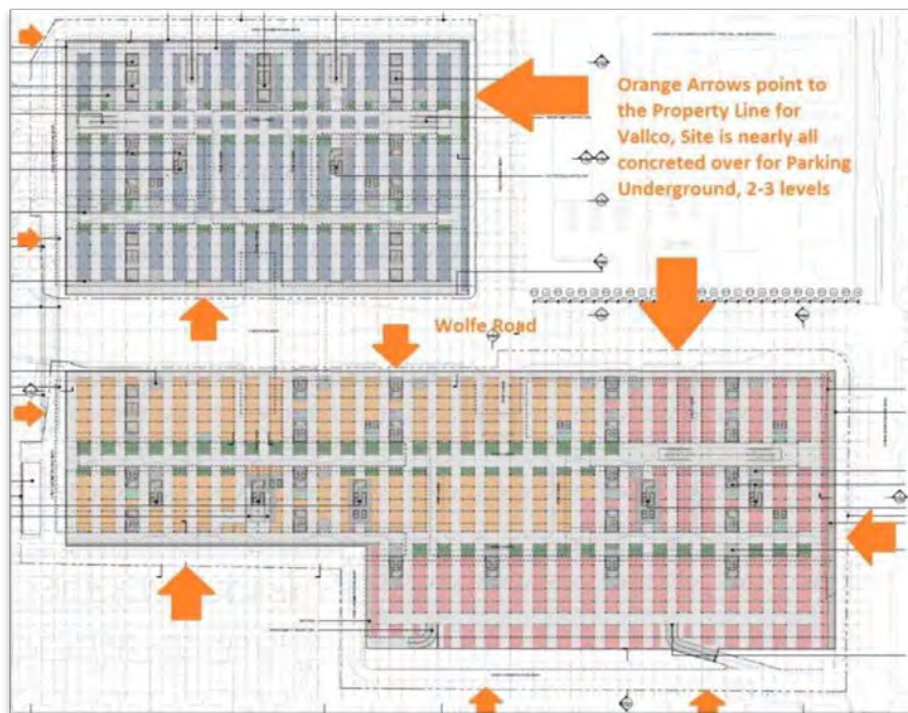
Figure 30: SB 35 Vallco Subterranean Parking Plan
