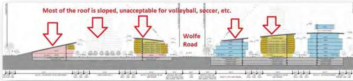
Figure 10: Section from SB 35 Vallco Application
