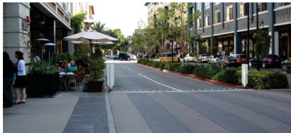
At-grade crossings with enhanced paving and detectable warning tiles
