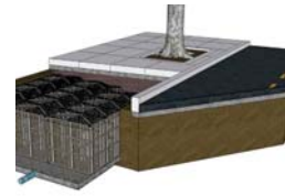
Geo-structure under pavements for enhanced soil profile and C3 Stormwater treatment
