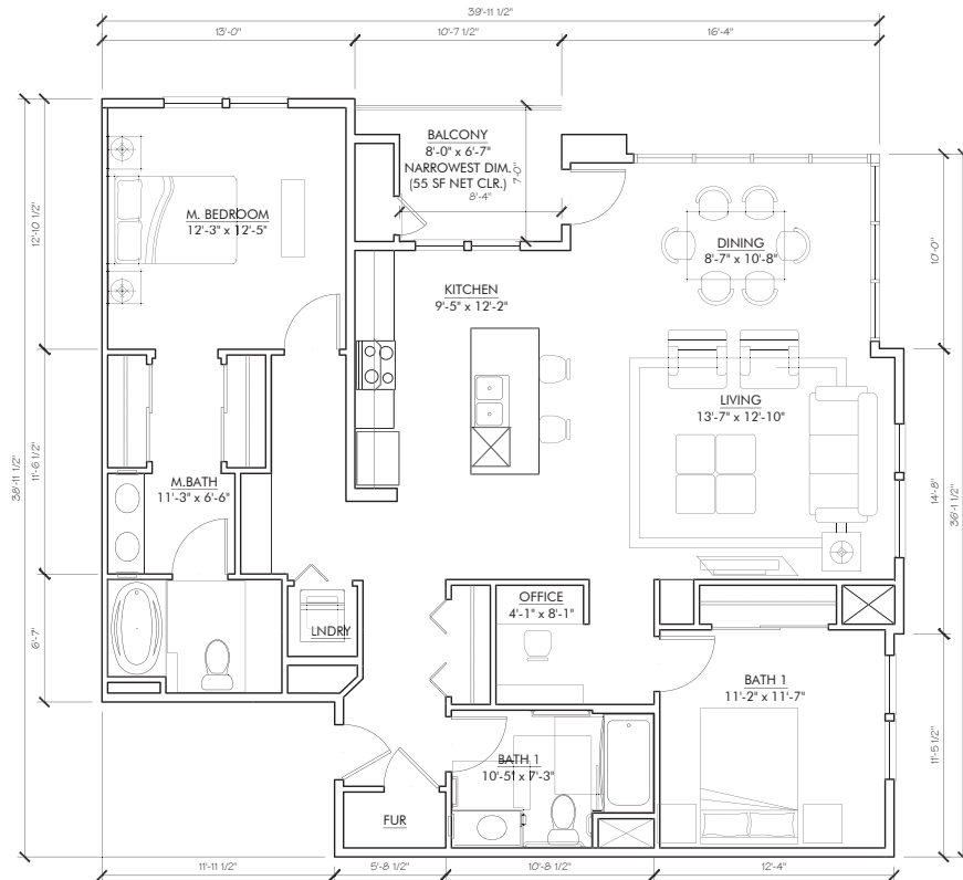
UNIT M1 (CORNER) (2) BED UNIT PLAN GROSS AREA: 1380 SQFT NET AREA: 1270 SQFT BALCONY: 55 SQFT
