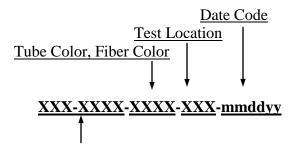
RAT (Reel Test) - Reel ID IAT (Installation Test) - Cable Segment FAT (Final Test) - End-to-End Location
