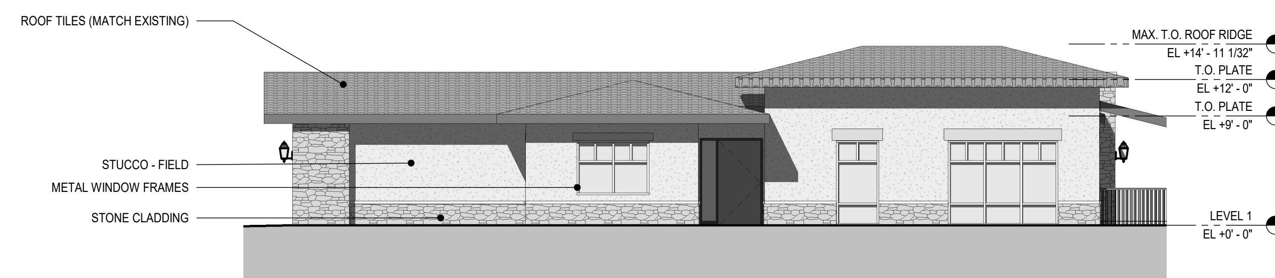
4 DUPLEX-SIDE ENTRY_SIDE PATIO - RIGHT ELEVATION - ILLUSTRATIVE SCALE: 1/8" = 1'-0"
