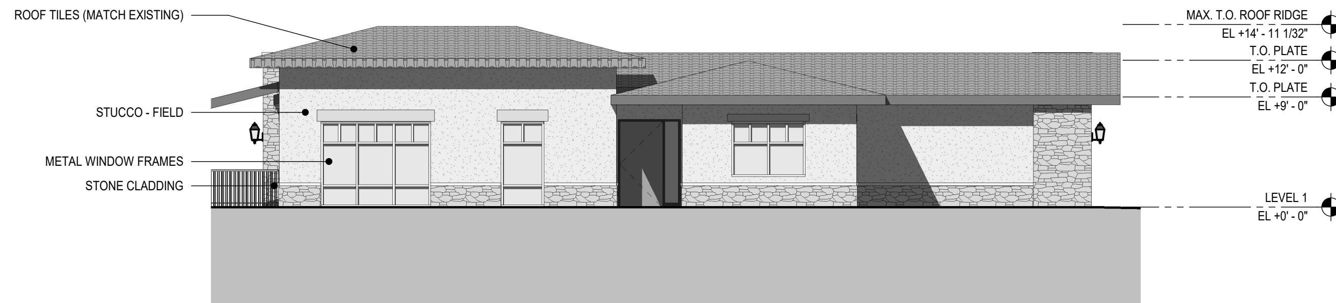
2 DUPLEX-SIDE ENTRY_SIDE PATIO - LEFT ELEVATION - ILLUSTRATIVE SCALE: 1/8" = 1'-0"
