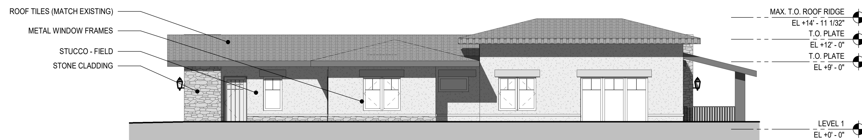
4 DUPLEX-FRONT ENTRY_REAR PATIO - RIGHT ELEVATION - ILLUSTRATIVE SCALE: 1/8" = 1'-0"
