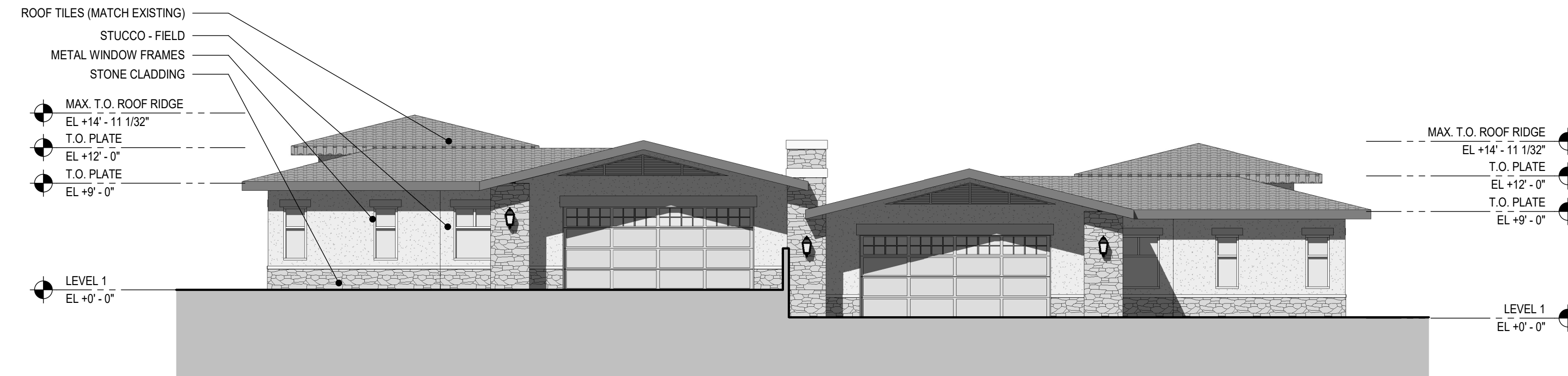
1 DUPLEX-SIDE ENTRY_SIDE PATIO - FRONT ELEVATION - ILLUSTRATIVE SCALE: 1/8" = 1'-0"
