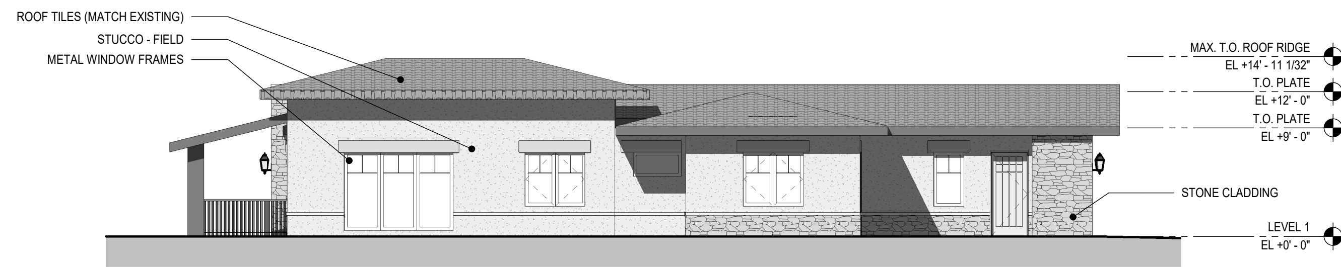
2 DUPLEX-FRONT ENTRY_REAR PATIO - LEFT ELEVATION - ILLUSTRATIVE SCALE: 1/8" = 1'-0"
