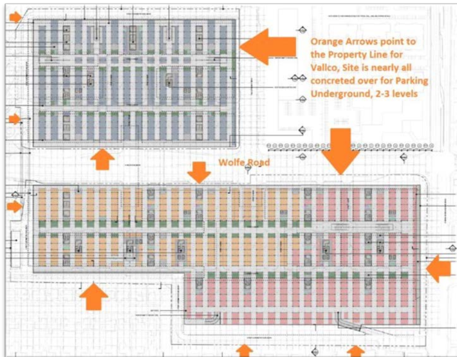
Figure 30: SB 35 Vallco Subterranean Parking Plan
