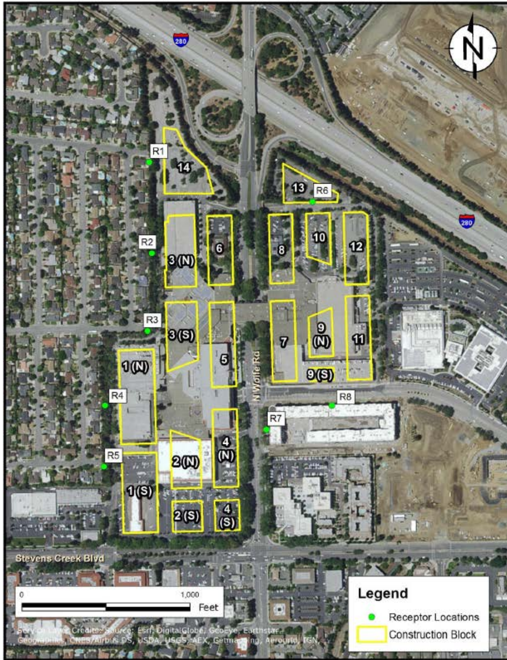
Figure 4. Construction Noise Receptor Locations
