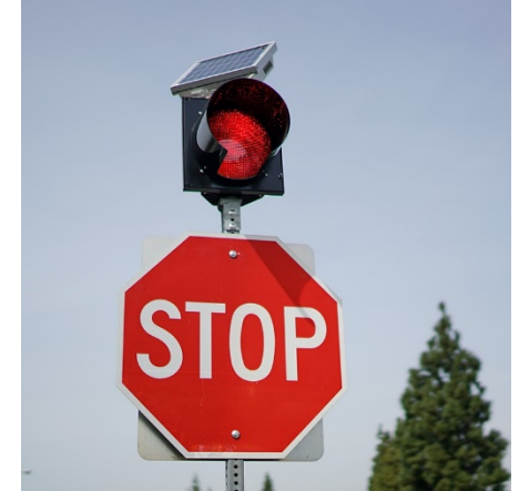
Install flashing beacons as advance warning
