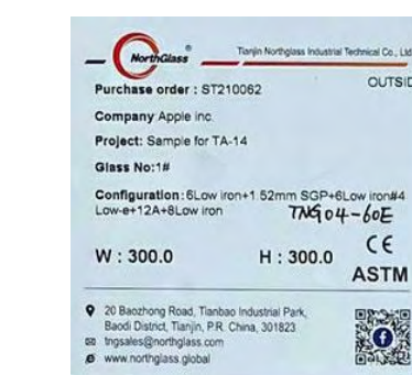
(GLT) TYPE: GLASS MANUFACTURER: NORTHGLASS PRODUCT: TN604-60E COLOR: CLEAR SPECIFICATIONS: IGU PROTECTED FINISH: SOLAR CONTROL COATING
