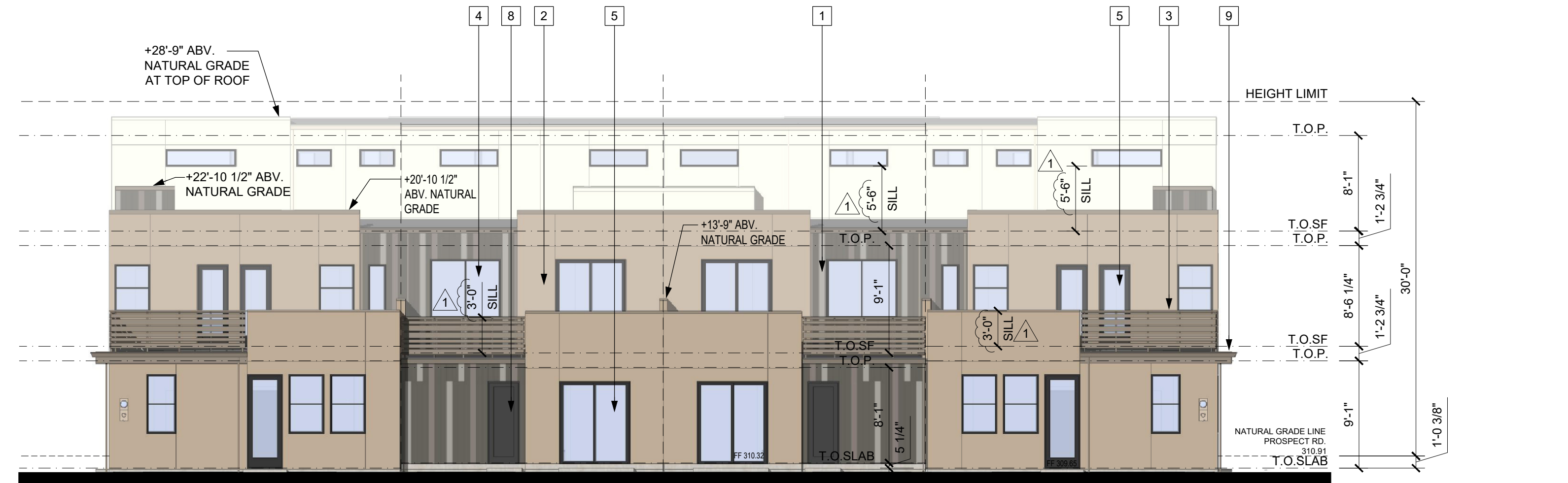
TH-3BR-B TH-3BR-A TH-3BR-A TH-3BR-B ALLOWED OPENINGS (X ≥ 3' F.S.D.): UNLIMITED (CRC TABLE R302.1(2))
