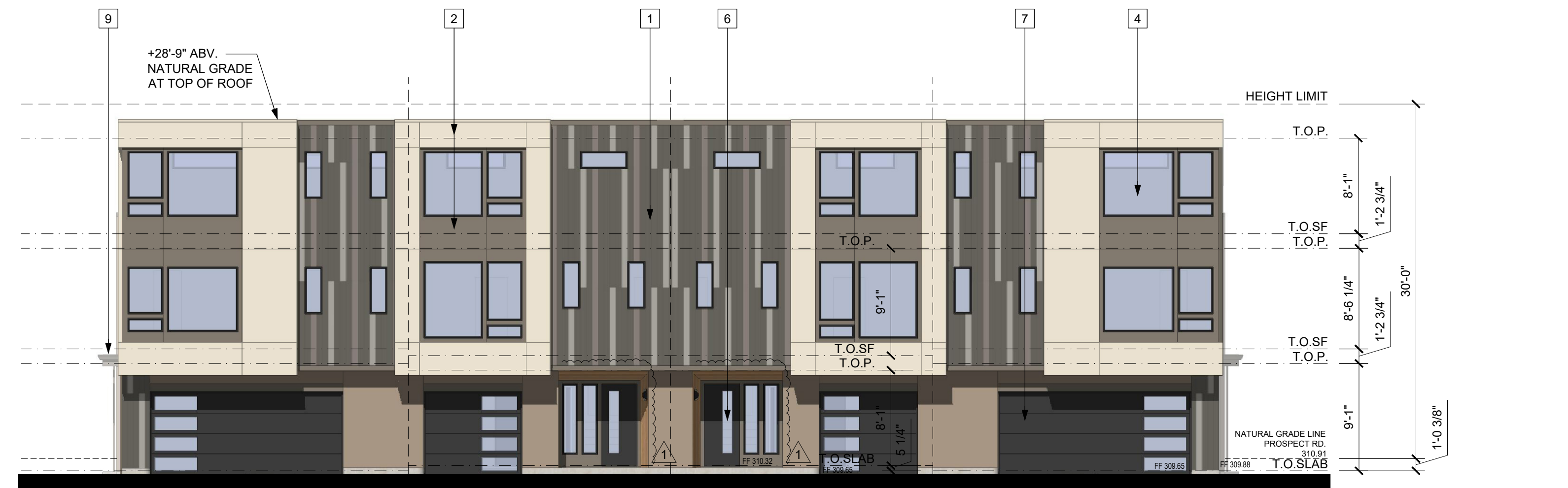
TH-3BR-B TH-3BR-A TH-3BR-A TH-3BR-B ALLOWED OPENINGS (X ≥ 3' F.S.D.): UNLIMITED (CRC TABLE R302.1(2))
