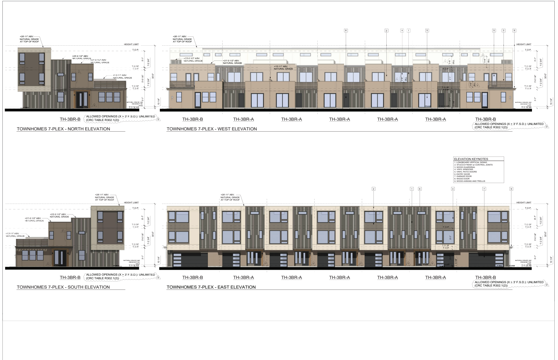
Figure 3-12 Townhomes 7-Plex Building Elevations
