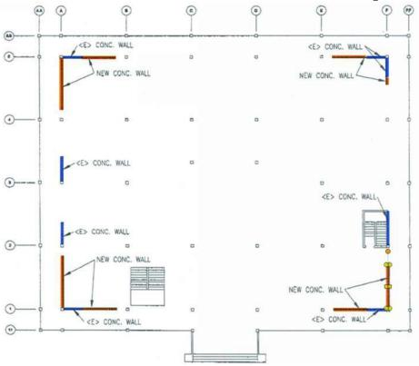
2005/06 Structural Analysis determined the need for additional shear walls, reinforcement of the existing shear walls, and improvements to the roof to lessen the loading and strengthen the diaphragm.
