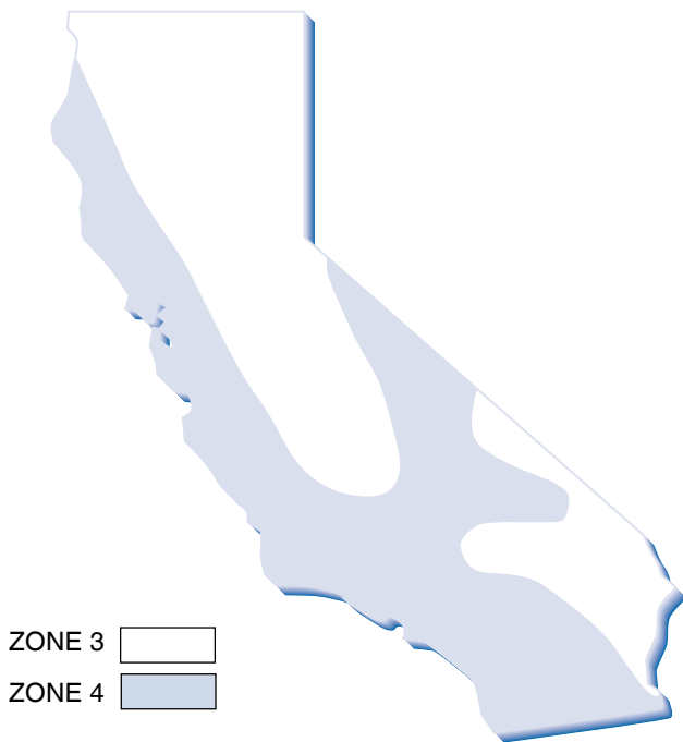
Figure 9—Seismic zones in California. All of California is in seismic zone 3 or 4 on U.S. Geological Survey maps. There are four zones; the higher the number the higher the earthquake danger. Stronger standards for buildings in zones 3 and 4 have been adopted in the Uniform Building Code.
