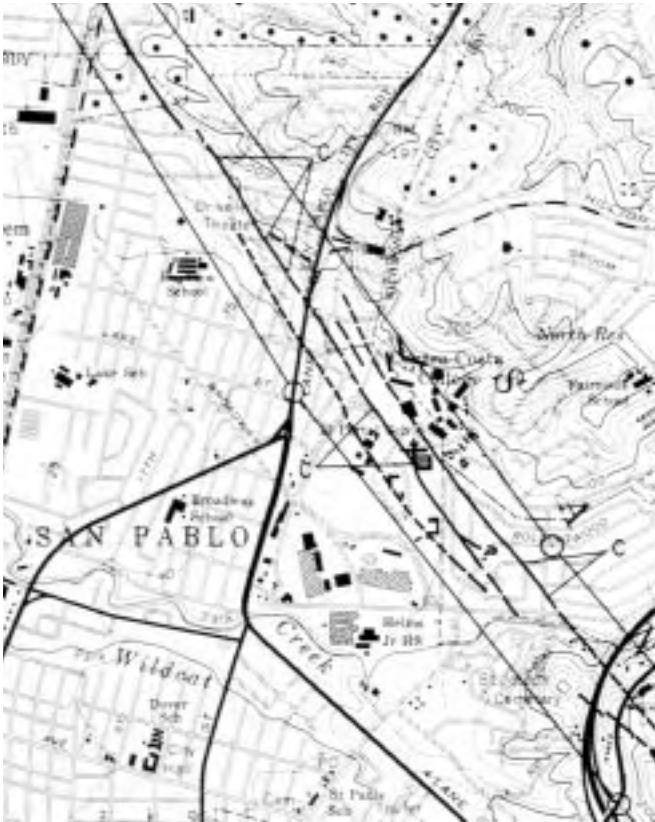
Figure 10—Earthquake fault zone map. This sample map shows the Hayward Fault as it runs through downtown San Pablo. The map provides an example of an Alquist-Priolo Earthquake Fault Zone that borders active fault traces in California.
